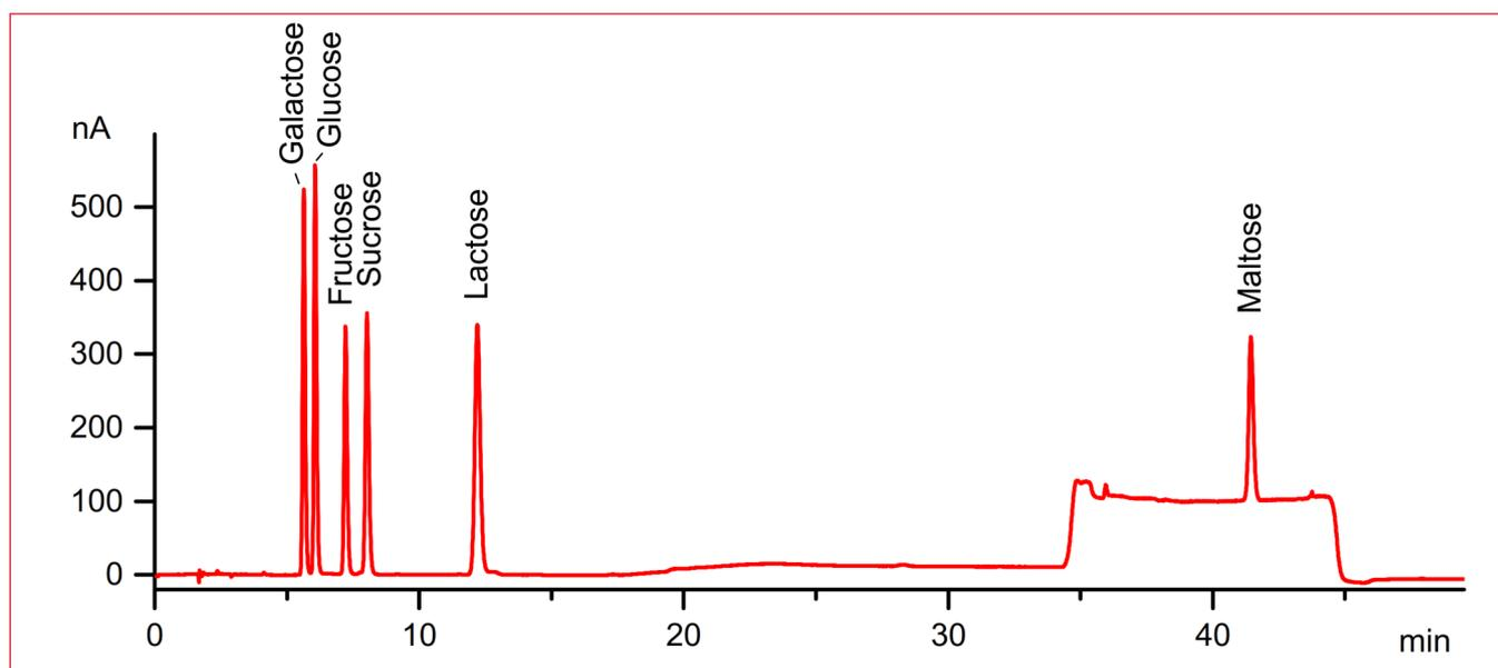
**Fig. 1.** Chromatogram obtained from an 10  $\mu\text{L}$  injection of 10  $\mu\text{M}$  galactose, glucose, fructose, sucrose, lactose and maltose in DI water. Separation was achieved using the LC-EC conditions and gradient program from standard GB5009.8—2023 shown in Table 1 and 2, respectively.
