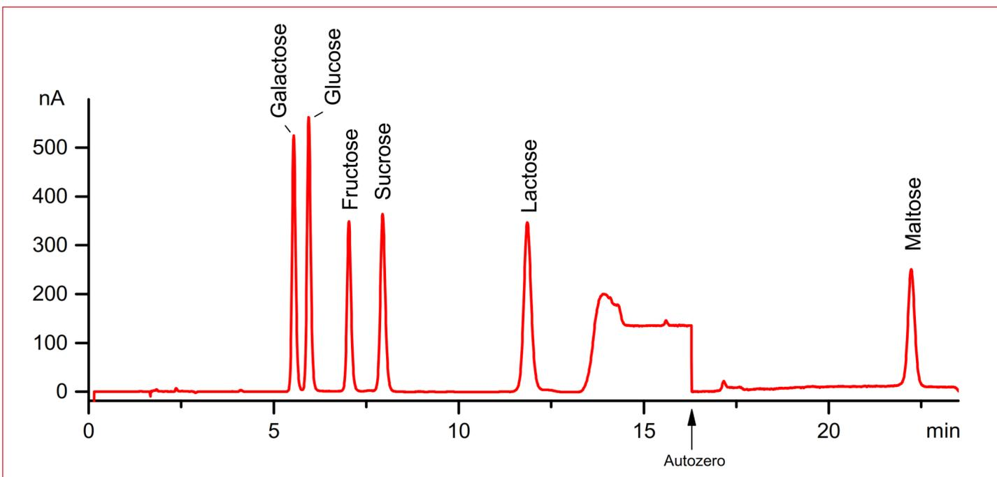
Fig. 3. Example chromatogram obtained from an 10  $\mu\text{L}$  injection of 10  $\mu\text{M}$  galactose, glucose, fructose, sucrose, lactose and maltose in DI water. Separation was achieved using the LC-EC conditions listed in table 1 and the adapted fast gradient program shown in table 2. At t=16.3 min an autozero was executed in the detector timed event table to zero the baseline prior to elution of maltose.
